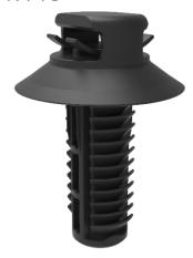
Cable strap adapter to be attached in a hole of a panel. Useful for big thicknesses (from 2 to 18mm.). Applicable for cable strap with thickness 1.3 to 2 mm and width 5 to 10 mm.
