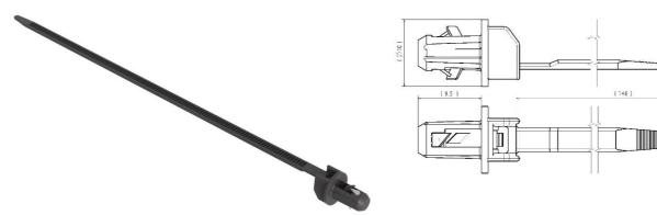
Cable strap to attach in a blind hole. Metal/plastic assembly with high retention force (min. 225N under  $23\pm5^{\circ}$ C). Applicable for hole in plastic diam.  $6\pm0.2$  mm deep min. 10mm.
