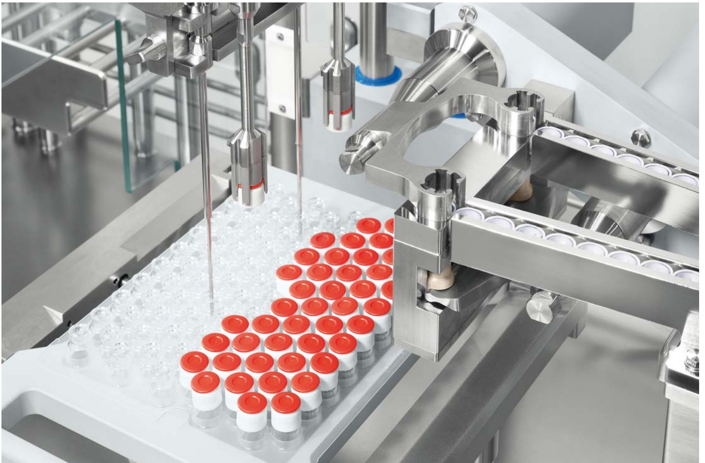
Filling and RayDyLyo® caps positioning on RTU vials.
