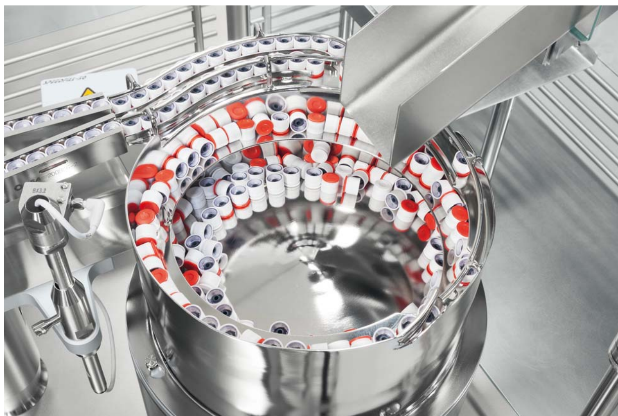
Feeding of different types of RayDyLyo® caps is done automatically, through AISI-316L vibrating feeders.
