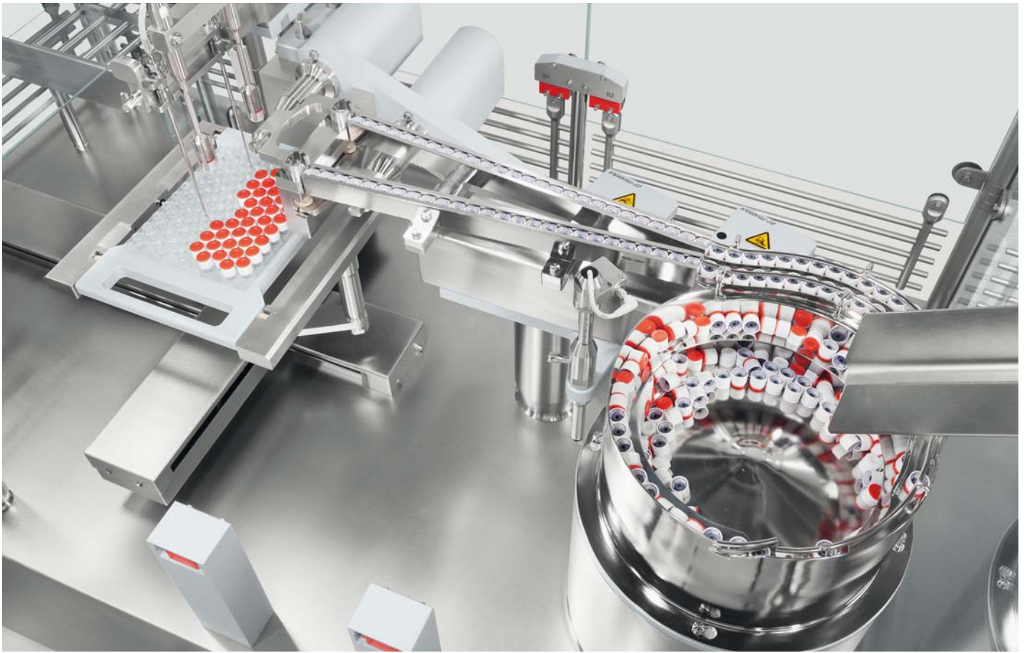
RayDyLyo® caps with pre-assembled stoppers are transported inverted to avoid any contact with the product, ensuring aseptic conditions.
