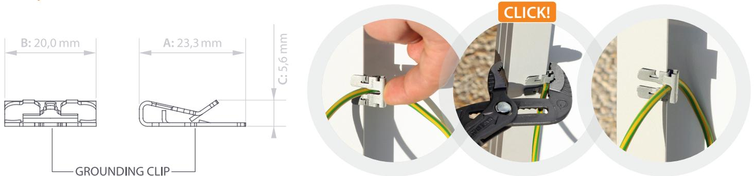
**Tool recommended:** Standard multigrip plier L250mm with self gripping teeth and locking button
