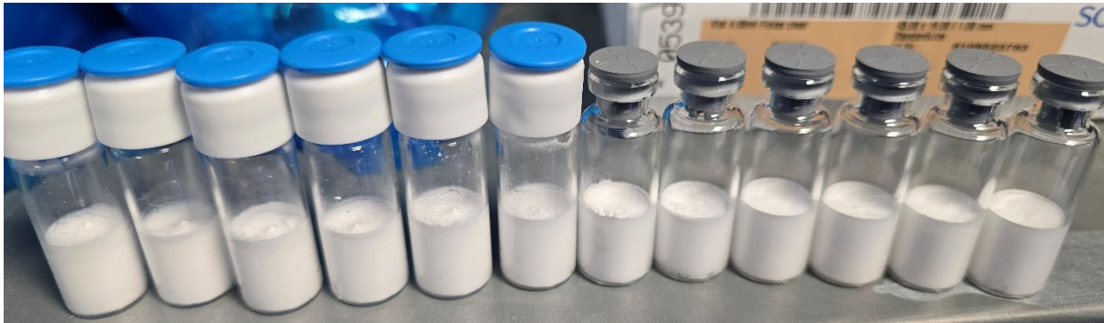
Figure 5: Comparison of 4R vials of conventional from test run 3 (right hand side) and RayDyLyo®
