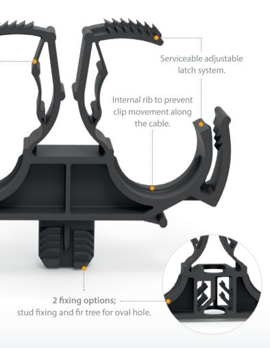
Manage a wide range of applications due to multiple diameters. Oval hole or stud fixing, single or double cable housing.
